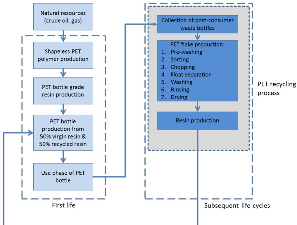
Figure 2-3 Bottle-to-Bottle Recycling System (adapted from Welle, 2011)
