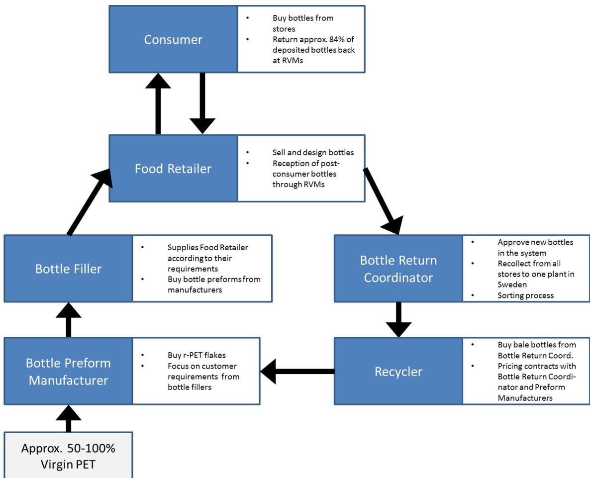
Figure 4-2 Current PET Bottle Recycling Operations in Sweden
