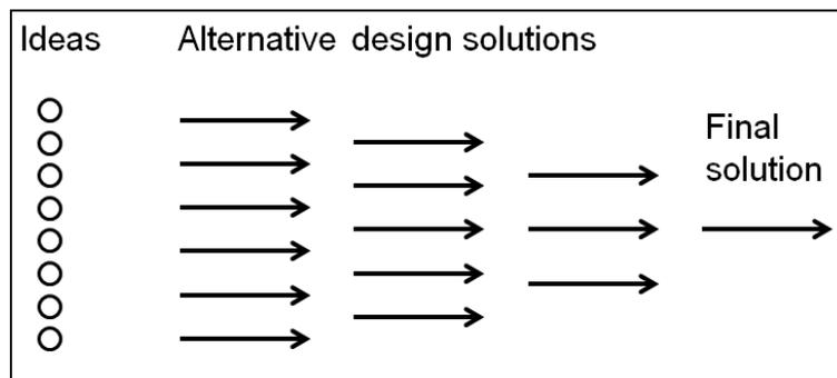
**Figure 1. An SBD process, inspired by Ward et al. [1995]. Design solutions are generated from ideas. Constraints are narrowed as knowledge is gained. Inferior solutions are eliminated and the process converges on a final design**
