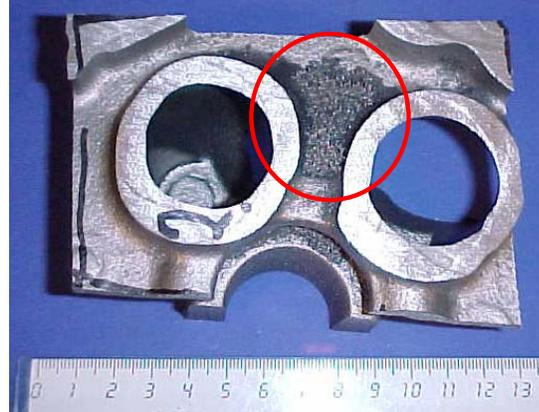
Figure 3. The investigated specimens showing metal expansion penetration.
