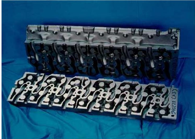
Figure 1. A sectioned cylinder head.
