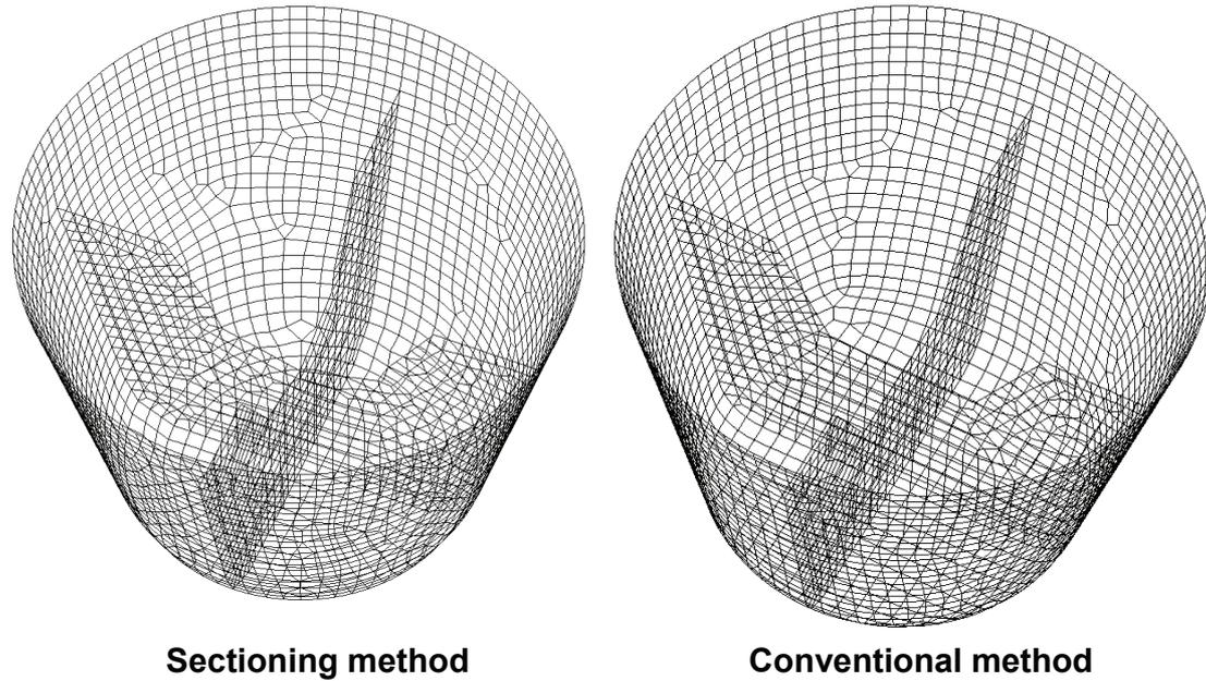
Figure 4: Shell element meshes applied to the target surfaces.
