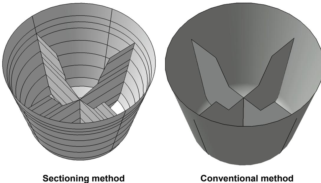
Figure 3: Resulting target surfaces.
