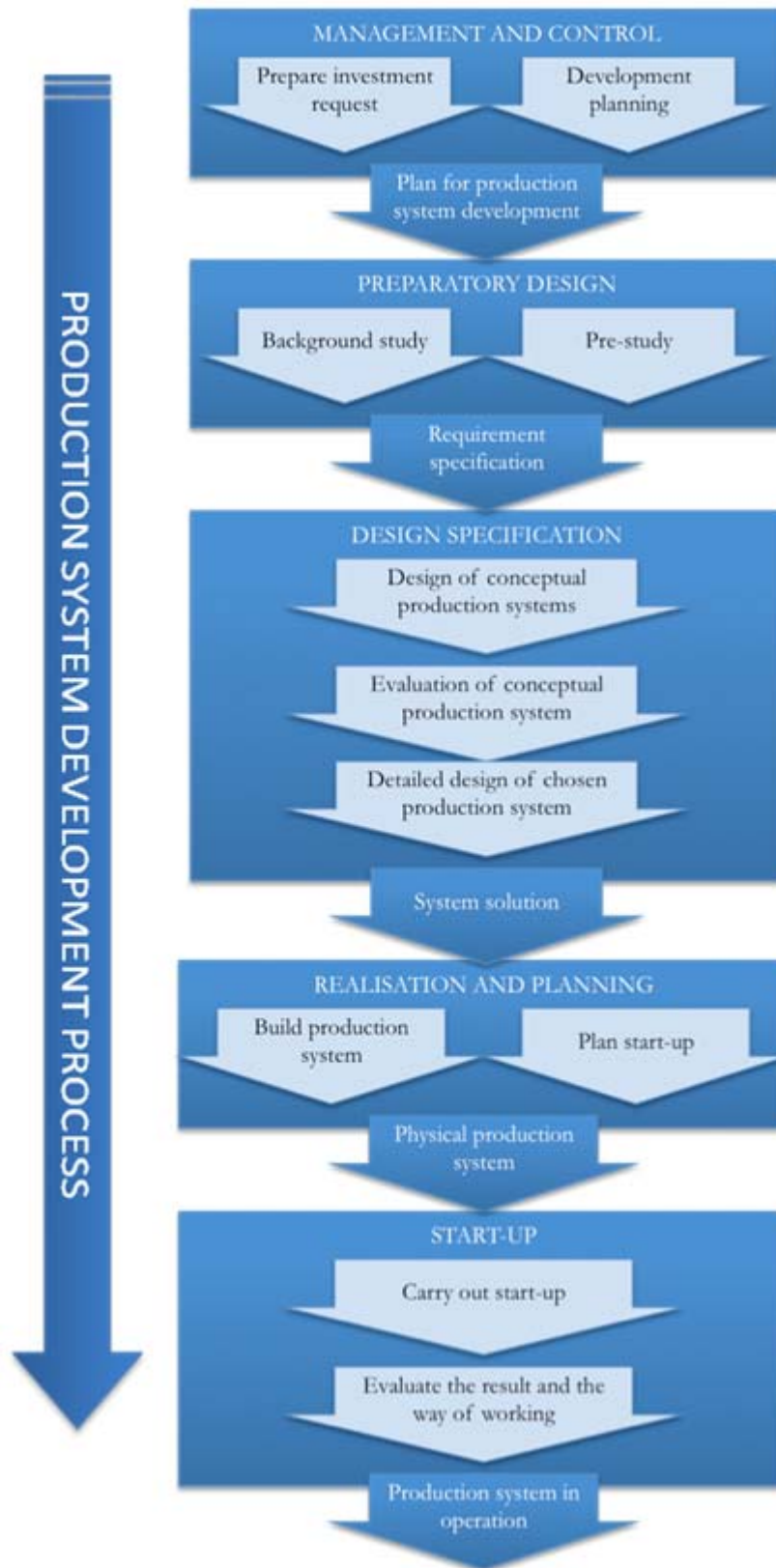
Figure 3. Production System Development Process. (Bellgran and Säfssten, 2002)
