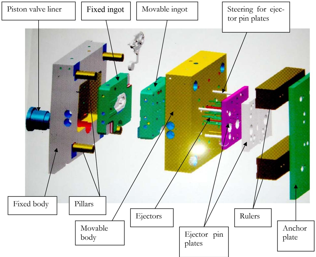
Figure 2-1 *The components of the casting mold*
