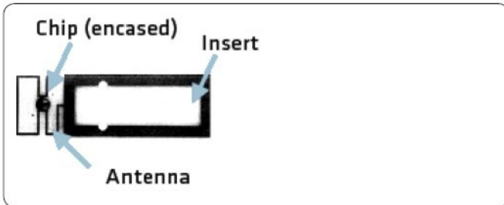
Figure 2 – Inlay RFID Tag components (Intermec, 2007)
