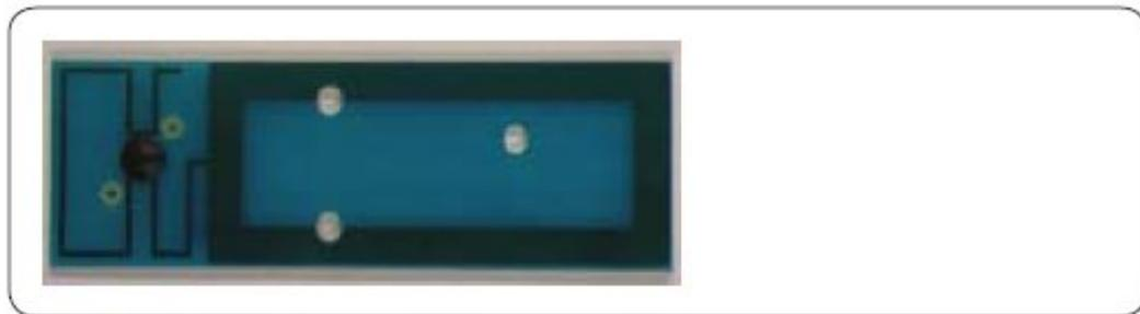
Figure 3 – Finished Tag (Intermec, 2007)
