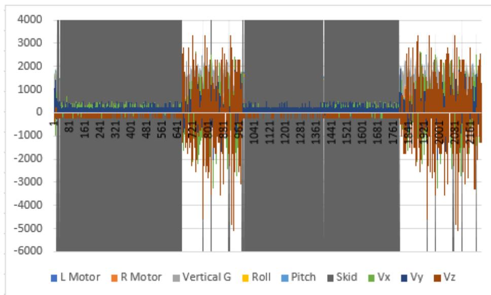
Figure 10. Graph showing prediction of skidding using motor currents and IMU signals after training session. Grey marks prediction of skidding and clear marks non-skidding.
