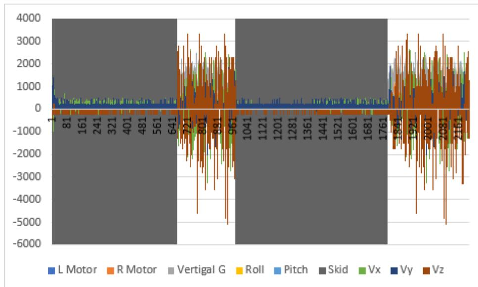
Figure 9. Graph showing training data with motor currents and IMU signals. Grey background marks skidding.
