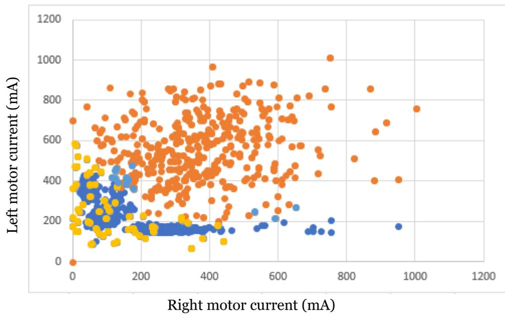
*Figure 8. Graph showing the incorrect predictions after training session due to overlapping scenarios. Yellow dots mark false detections and light blue dots marks missed detections.*
