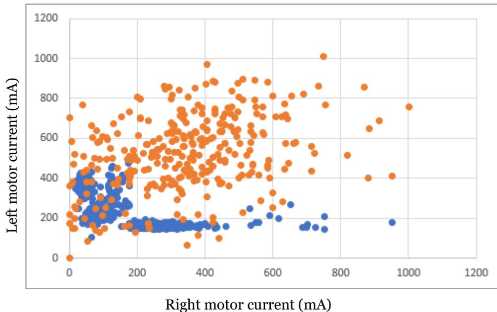
*Figure 6. Graph representing collected data of motor currents. Orange represents non-skidding and blue represents skidding.*
