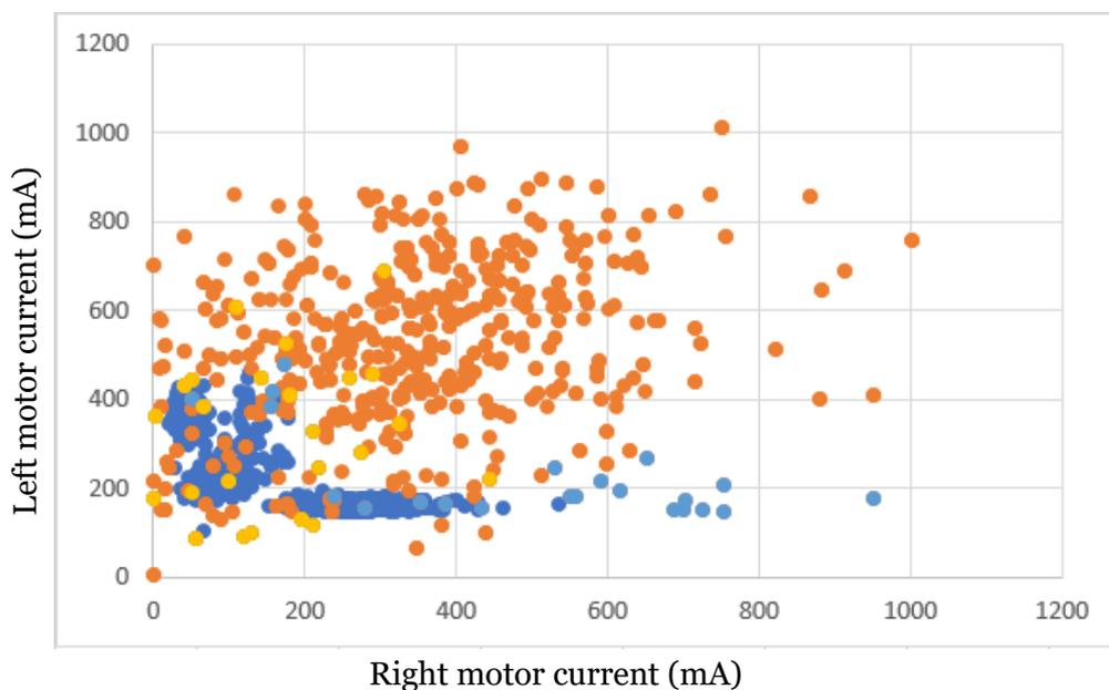
Figure 11. Graph of motor currents representing the predictions with IMU for comparison. Yellow dots mark false detections and light blue dots marks missed detections.
