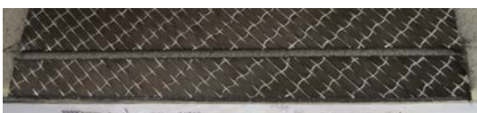
Fig. 21 The cutting result when cutting a stiff preform with a 120 degree chamfer angle using Test Setup 2
