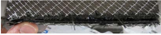
Fig. 20 A look into the cut generated when cutting a less stiff preform using Test Setup 1
