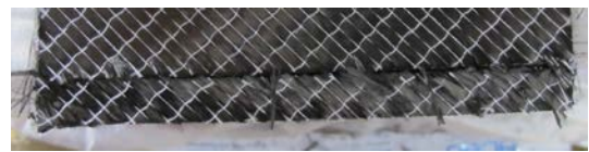
Fig. 19 Cutting result for a less stiff preform without cutting support under the cutting line
