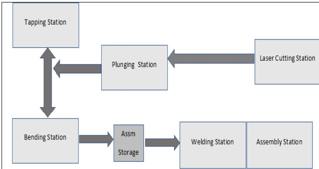
Figure 4.1 represents the diagram of a production layout that indicates the material flow from laser cutting station to the final assembly station. The original layout map cannot be used for external purposes as per company's rules and regulations. Hence, a diagram like a layout was drawn to increase the understandability for the readers.
