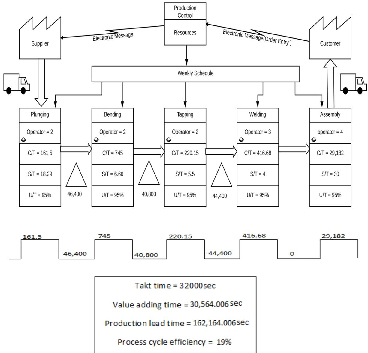
Figure 4.6 As-Is state analysis Value Stream Mapping
