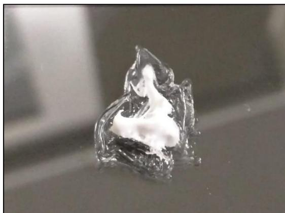
**Figure 22: Pluronic scaffold obtained by inkjet printing.** Unsuccessful printing the support structure using Pluronic and then printing the OsteoInk. The Pluronic was not able to support the OsteoInk.
