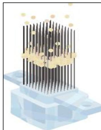
**Figure 7: Needle block ('Kenzan') for scaffold free biofabrication:** A robotic arm controls the placement of cell spheroid on this microneedle array [25]
