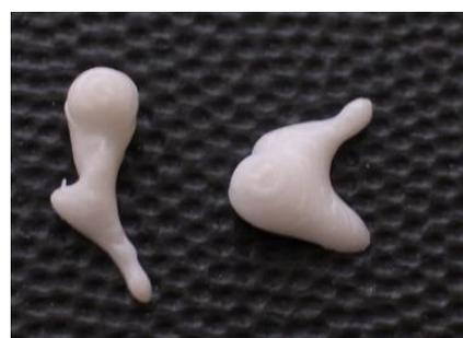
**Figure 18: Printed malleus and incus after curing for five days.** No discernable changed in structure or exterior texture observed.
