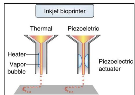
**Figure 6: Example of a 3D bioprinting with inkjet method.** Thermal and piezoelectric. [20]
