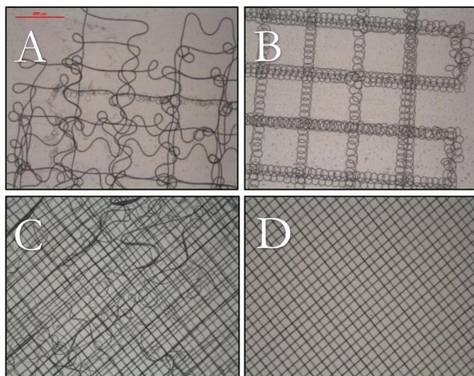
**Figure 23: MESW visualized with stereomicroscopy. (Red bar for scale: 500  $\mu$ m) A:** Initial print with fan. **B:** No fan and low feed rate. **C:** High feed rate and high collector plate distance. **D:** High feed rate and low collector plate distance. Red line (500  $\mu$ m) for reference.
