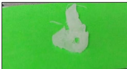
**Figure 21: PCL scaffold attempted through extrusion printing.** Individual PCL Support structure printed on adhesive backed material. Glass slide was not able to be used for this print.
