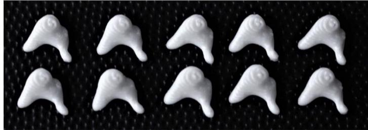
**Figure 19: Repeatability prints.** The ten incus prints after curing. Size and texture are repeatable though minor differences in external texture can be noticed.
