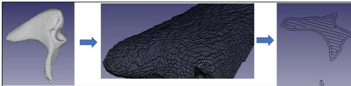
**Figure 4: Example of 3D model (ossicle) processing.** The initial model is processed into a mesh which is then transformed into specific printer path with infill. The rightmost frame shows a single layer that bioprinter will create.
