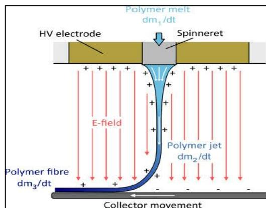
**Figure 8: MESW method.** The molten polymer is fed through a spinneret due to pressure. The HV electrode (including spinneret and melt) becomes charged and the collector becomes a ground. This draws out the polymer in a Taylor Cone formation. The collector plate directs where the polymer effectively “writes.” [28]
