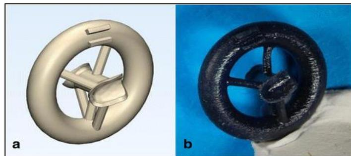
**Figure 3: Proposed 3D printed polymer based individualized implant.** CAD model on the left (a) and printed part on the right (b) [13]
