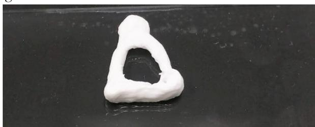
**Figure 13: First successful print with the regenHU printer.** The object is oversized compared to a human stapes and many details seen in the virtual modeling of the stapes are not evident in this print.
