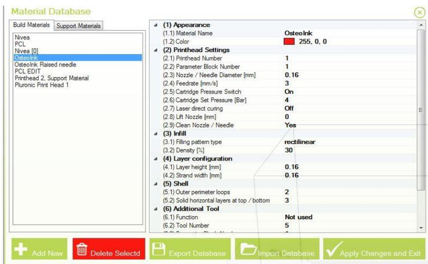
**Figure 14: Final Settings for printing OsteoInk.** Nozzle Diameter, feed rate, pressure, filling pattern, density, layer height, strand width, outer perimeter loops, and solid horizontal layers at the top/bottom were updated. Lift nozzle was attempted. Screenshot taken from regenHU's BioCam software. The baseline settings were taken from NIVEA crème and then optimized through experimentation.
