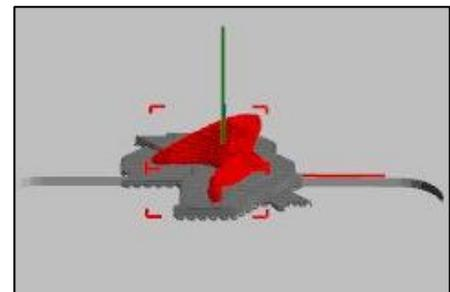
**Figure 20: Design of an ossicle support structure.** Red color represents the model while the grey area represents the support structure created in BioCAM.
