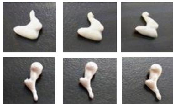
**Figure 17: Three completed prints of the malleus and incus on a glass slides before curing.** Support structure was not used as layers were omitted from the print to obtain a flat base. The desired structure and the proper external texture were achieved.
