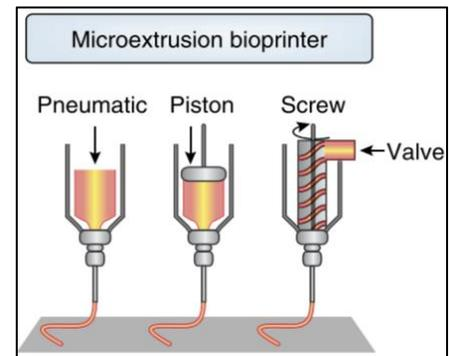
**Figure 5: Example of 3D bioprinting with extrusion.** Three types of extrusion methods are shown. Pneumatic and piston are the most common. [20]
