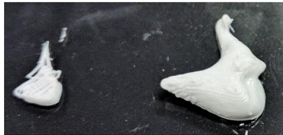
**Figure 16: Infill prints.** The left shows the rectilinear interior fill pattern while the right shows the completed print of an incus. Printed in OsteoInk.
