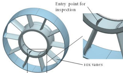
Fig. 3. Static turbine frame
