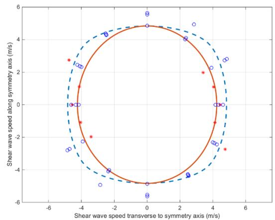
Figure 1(c): PT (red) and QT (blue) theoretical propagation modes compared with the velocity estimated using one (red asterisk) and two (blue circles) probes.
