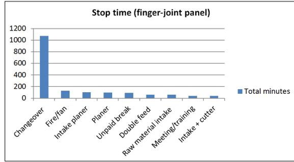
Figure 2. Stop time for finger-joint panels.
